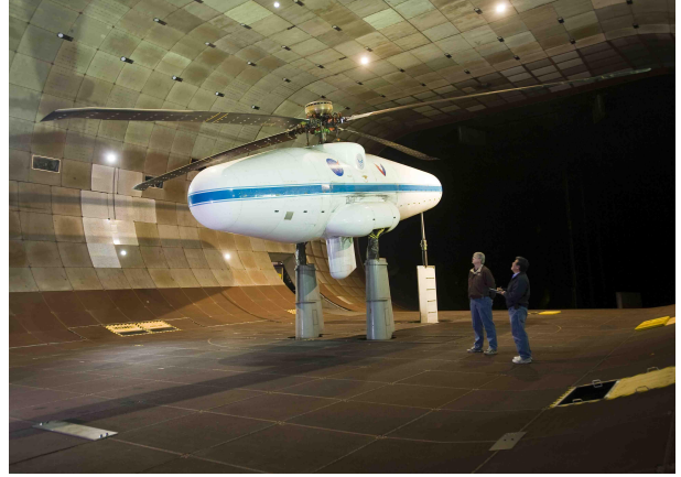
Figure 1 – UH-60A airloads rotor in NFAC 40- by 80-Foot Wind Tunnel.
